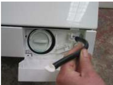
If a pipe like this is fitted to your machine, pull the stop from the end of the pipe, and drain the water that is left in the machine into a suitable container. This will save you getting water on your floor, when you remove the filter. Even if the machine has pumped the water out, there will always be some water left in the sump. Always refer to manufacturer's handbook.
